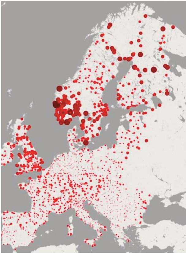
Figure 12 Largest GICs measured in Europe, 1996-2008 (source: EURISGIC project)
